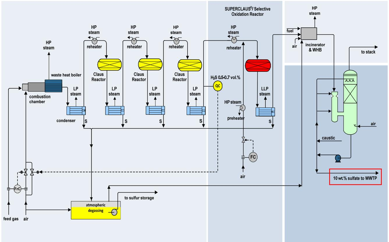
Figure 1: Line-up of SRU with SUPERCLAUS® + Caustic Scrubber
