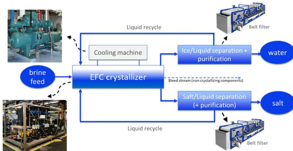
Figure 5: The Process Flow Diagram of the EFC process showing the main components
