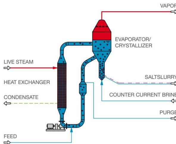
**Figure 4: Forced Circulation Crystallizer (FCC)**
