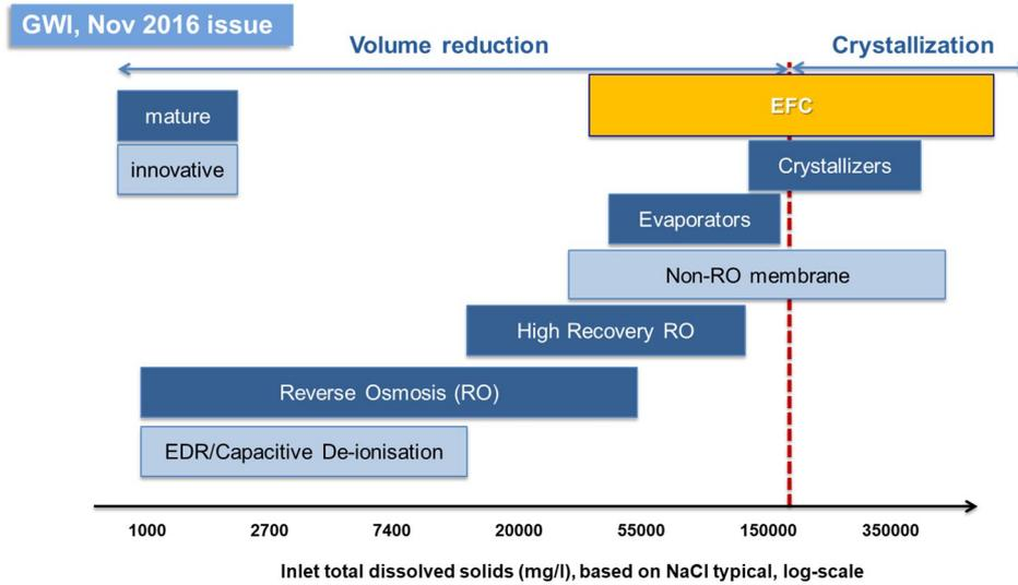
**Figure 3: Volume reduction and crystallization technologies for saline solutions**
