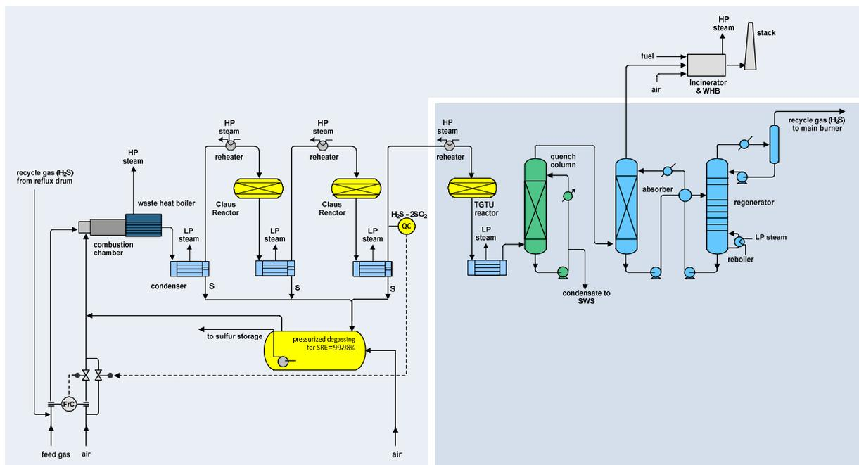
Figure 2: Typical SRU with amine based Tail Gas Treating technology
