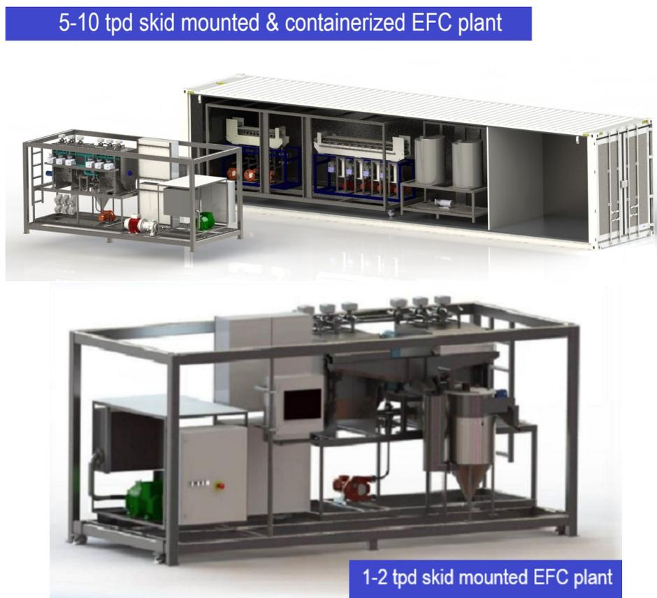
Figure 6: Examples of modular EFC treatment skids
